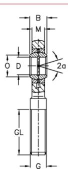
A = 82 a (degrees) = 6 B = 25 D = 35 Dynamic drive (kN) = 80 F = 140 g = M36x3 GL = 82 L = 181 M = 21 O = 39.8Static drive kN = 144
